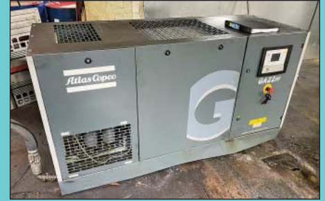
30 HP Atlas Copco Air Compressor w/ Built in Dryer
